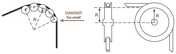
Don't confuse the diameter of the sheave with the radius. The radius MUST match the cable's bending radius.
